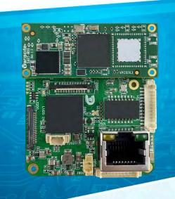
**Blue Mamba Neo** IP video encoding module has been specifically designed for compact embedded vision systems.
