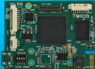
*Twiga has designed the first LVDS to analog HD & analog SD interface board for Sony FCB-EV7520, FCB-EV7520A and new Sony FCB-EV9500L.*
