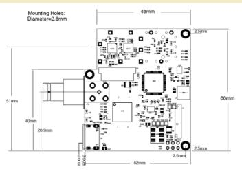
Maximum bottom component height = 11.0mm (SFP cage) Maximum top component height = 11.0mm (BNC connector) PCB thickness = 1.5mm
