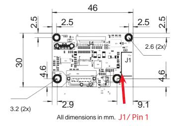
+ Max. component height = 10.5mm (HDMI connector, J2)
